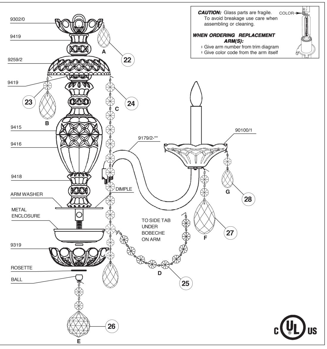
20 Install arms into washer. Line up holes in arms with dimple in washer. Use lock washer and nut to secure arms in place.
