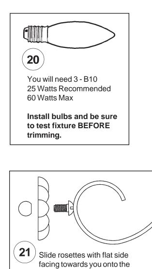
screws and secure with balls
