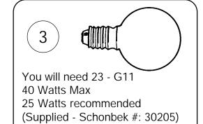
Install bulbs and be sure to test fixture BEFORE trimming.
