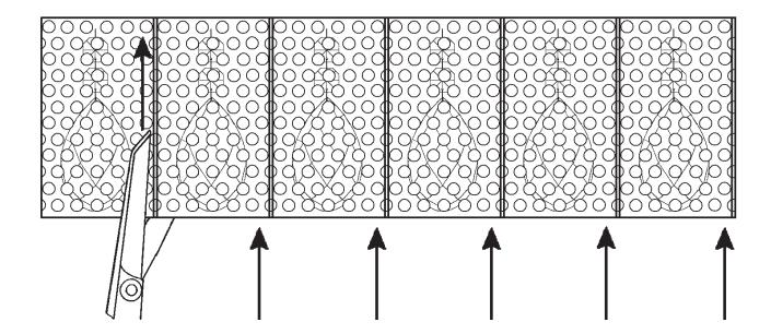
**NOTE:** Work on one crystal set at a time. Follow the black line from top to bottom according to the numbered steps on the trim diagram.
