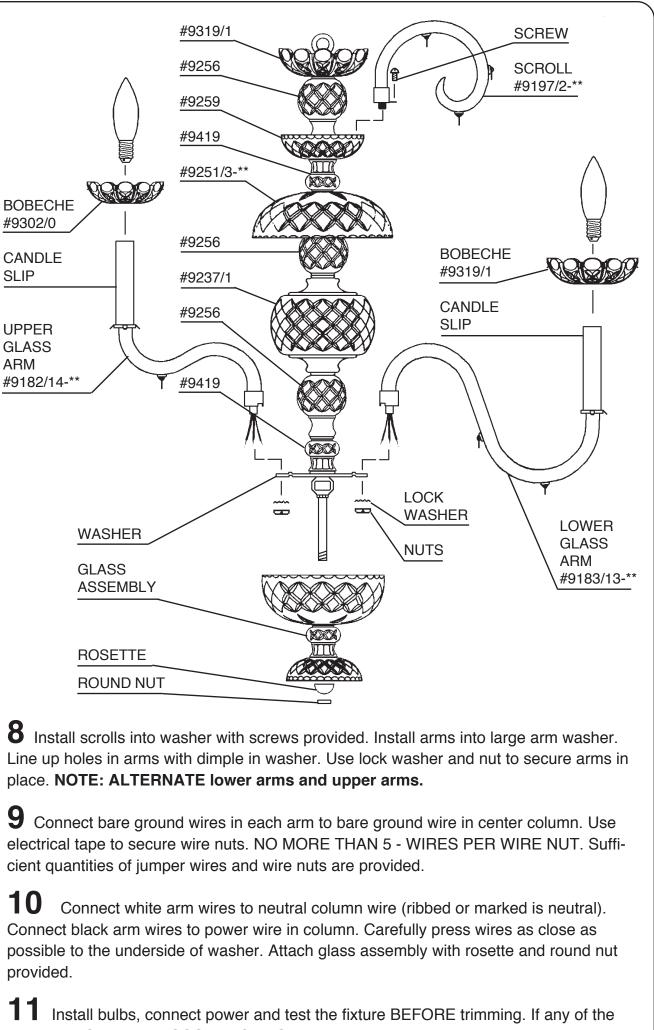
bulbs do NOT light - DISCONNECT POWER. Double check the wire connections.
