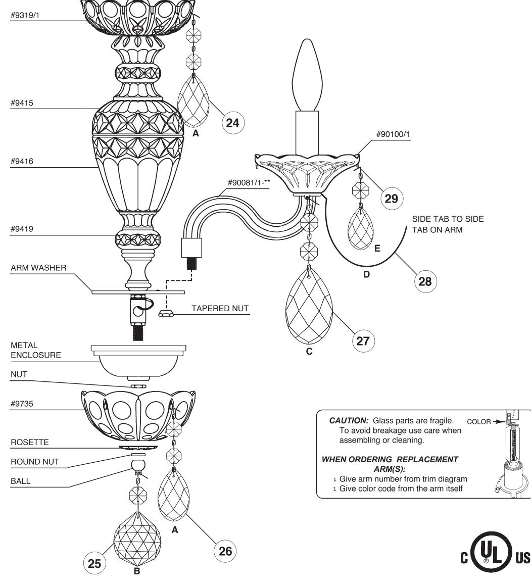
(22) Install arms into the holes on the washer. Line up holes in arms with dimple in washer. Use lock tapered nut to secure arms in place.
